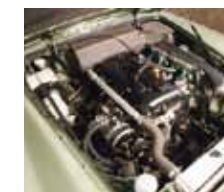
Above: alloy 2-litre ‘four’ and six-speed ‘box’ are by Mazda. Right: Twin-Cam MGA-style alloy wheels
